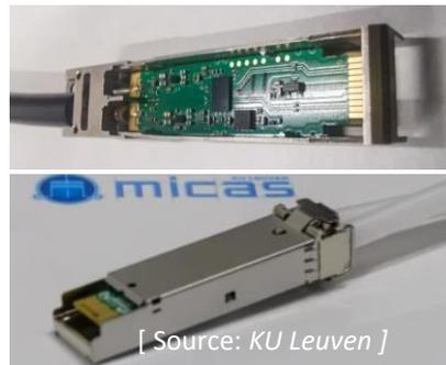
SFP28 module with 135 GHz CMOS radios targets replacement of optical modules in data centers
