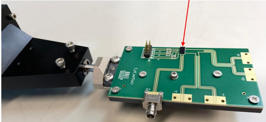
3D printed PCB holder, designed to be mountable to a commercial probe-station manipulator for fine alignment with PMF on  $\mu\text{m}$  scale
